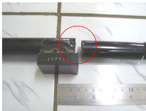
Figure 2. As receive condition of failed lateral control rod
