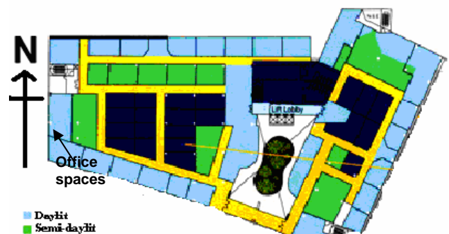
Figure 3: The interior space layout of LEO Building shows the office areas are designed along the facades to maximise the use of daylight. It is L-shape on plan with and the main facades are facing north and south.
