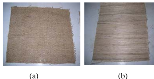
Fig 4 : camera image of preform : (a) woven ; (b) unidirectional-UD
