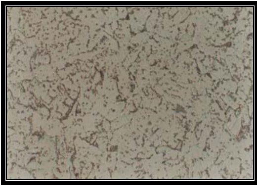
Figure 5. . Prior Austenite Grain Boundaries saturated ,picric 10% acid etching,,sample no 1,500x Magnification
