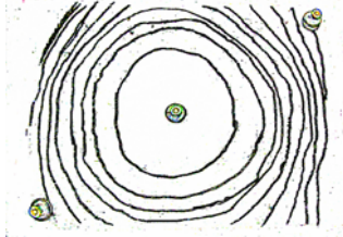
Fig 8 : Image view resin flow of Diagonal port . (the curve line refer to front flow for each minute , dimension 29x34 cm) by measuring wetting area incrementally we could tabulate the data as given in Table 1 and fig 8.
