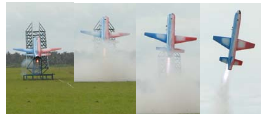
Figure 15. The dummy HSFTB tends to produce roll-yaw coupling to the right side of the fuselage
