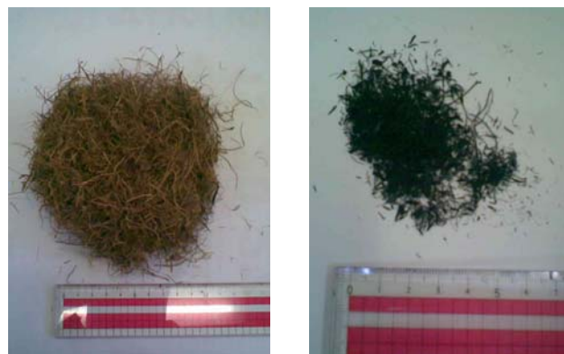
Figure 3: Photos of the palm fiber basic material (left), after being carbonized (right).
