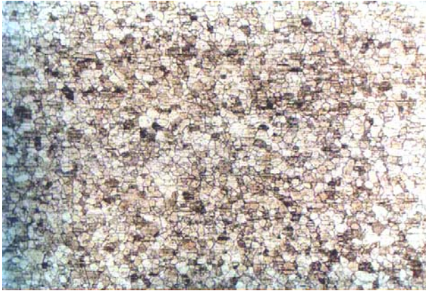
Figure 6. Microstructure in base metal of rod, mag 100X, 2% Nital etched, consist of ferrite and small amount pearlite
