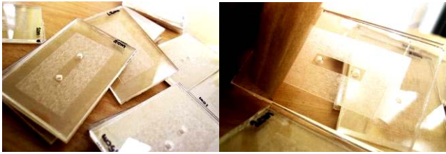
Figure 4. Photographs of the customarily microfluidic chips made by using double-sided sticky tape that are used in this experiment.
