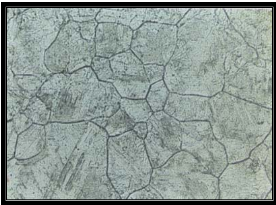
Figure 11. Prior Austenite Grain Boundaries saturated Picric Acid 30%, sample no 3,100x Magnification
