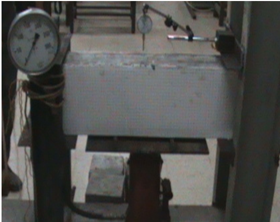
Figure 4 : Third point flexural test setting ([3]-[6])
