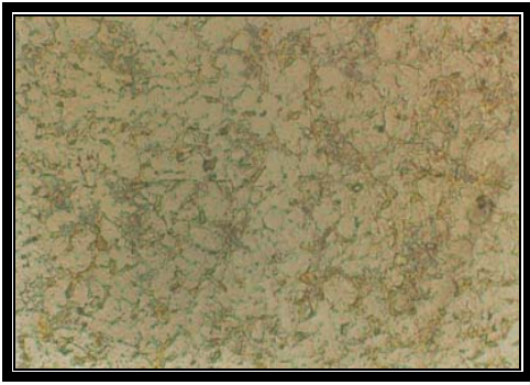
Figure 5. . Prior Austenite Grain Boundaries, Modified super picral etching ,sample no 1,500x Magnification
