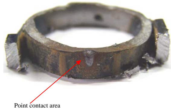
Figure 5. Point contact between the rod and mass dumper, notice the bright appearance and slightly deformed
