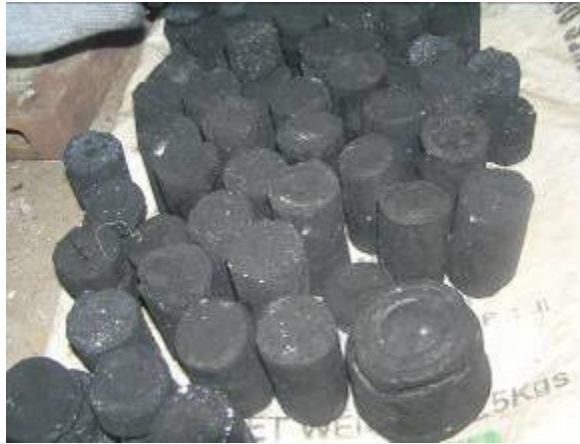
Picture. 2. Pellet with diameter of 3cm, and high of 6cm.
