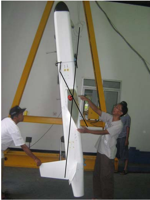
Figure 18. Manual method photometry to discover the c.g location
