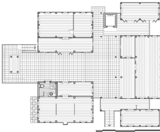
Figure 5. Main floor plan of Thai house shows modularity of house units.
